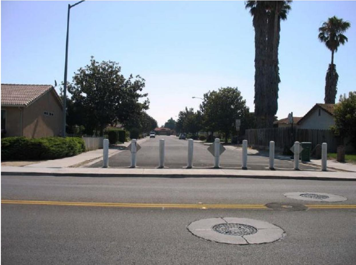
Full roadway closures are created with the placement of a physical barrier to block all vehicle traffic. Pedestrian and bicycle traffic are usually unrestricted.
